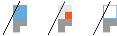
Figure 8: On the left, a view ray hits the blue octree node which should be refined. In the middle, the children of the blue node are highlighted in red. As all children are invisible, we mark the blue node for occlusion rendering only in the next frame.
